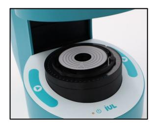
Push the Run button on the bottom right: . The instrument will proceed to perform several image captures, and finally, an image of the calibration disk will appear on the Image Panel.
